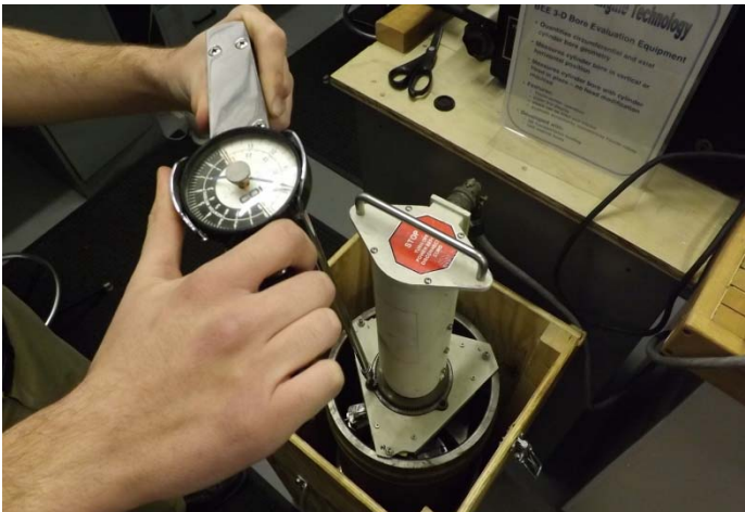
BEE 3-D is inserted and the top clamp tightened in the bore
