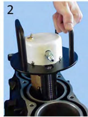
Replicator head is inserted into bore
