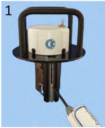
Replicate material is dispensed into replicate bar
