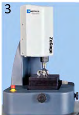
SEE-3D replicate is examined with interferometer
