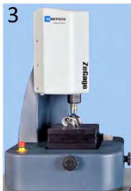
SEE-3D replicate is examined with interferometer
