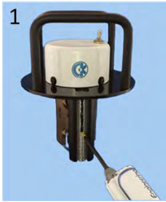
Replicate material is dispensed into replicate bar
