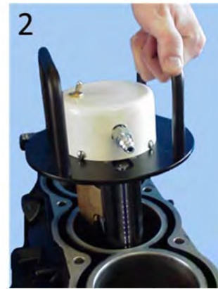
Replicator head is inserted into bore
