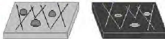
Replicate material is removed from surface producing a negative copy of the surface
